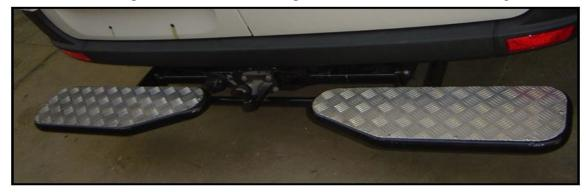
Secondly, it is possible to mount a coupling system together with an additional step. This step can turn away when it touches the drawbar in the curve.
